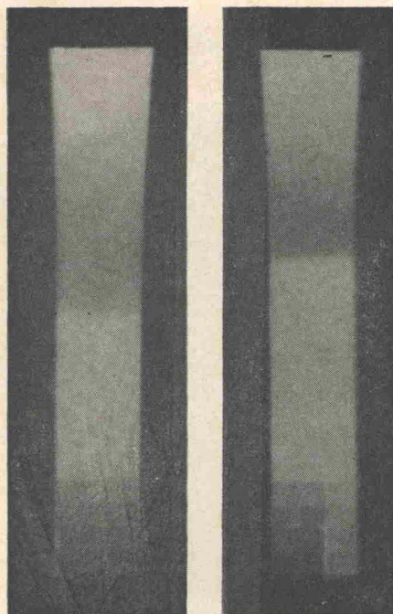
FIG. 12. Radiographs of detonation in one-dimensional channel flow for mixes G (left) and C (right). The aluminum "step wedges" are visible in the lower parts of the radiographs. The detonation is proceeding in both cases from top to bottom. The radiographs illustrate the relatively small expansion of the stream tube with this confinement.
